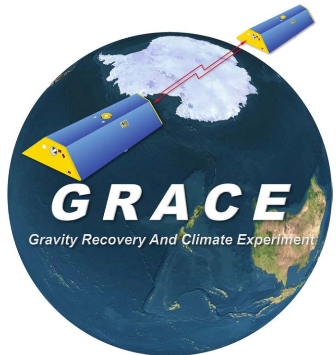
Fig. 2. The Gravity Recovery and Climate Experiment (GRACE) is a twin satellite mission orbiting the Earth at an initial altitude of about 500 km in a polar orbit ( 89^\circ inclination), and 220 km apart. GRACE was launched on March 17, 2002, with a designed lifetime of 5 years. Now entering its 8th year the GRACE mission has been extended to 2012 or beyond. GRACE utilizes a state-of-the-art technique to observe variations of Earth's gravity by tracking the inter-satellite range and range-rate between two coplanar, low altitude satellites via a K-band ranging (KBR) system. In addition, each satellite is equipped with a SuperSTAR Accelerometer, GPS receiver/antenna, Star Cameras, and Laser Retro Reflectors to complement the science instruments. The GRACE Science Data System uses the range and range-rate data, along with ancillary data, to estimate a new gravity field every month, which can be used to study mass redistribution within the Earth system.
